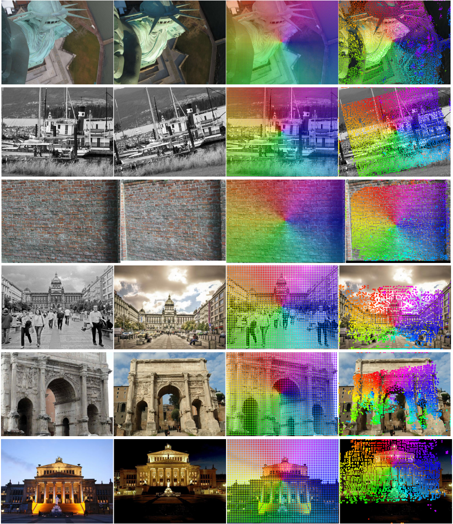
Fig. 2: Dense Correspondence. For each row, the first two columns show original images, and the last two columns show the correspondences found by our method. Colors indicate correspondences. The first and second three pairs of images are from HPatches [1] and MegaDepth [8], respectively. For each query point in the first image, we find its correspondence in the second image by nearest neighbor search using our dense descriptors. For the ease of visualization, we show correspondences for query points with an interval of 50 pixels on regular image grids.
